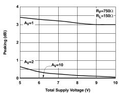
Peaking vs Supply Voltage for Inverting Gains
