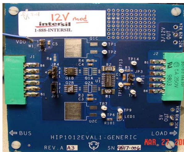
FIGURE 37. +5V AND +12V EVAL BOARD PICTURE
