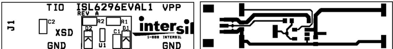
FIGURE 20. LAYOUT OF THE EVALUATION BOARD (SILK SCREEN AND TOP LAYER). THE BOARD DIMENSION IS 1CM X 4CM.
