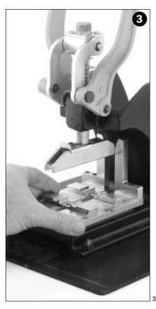
Install the 10981-5 platen and the locator plate on the press.
