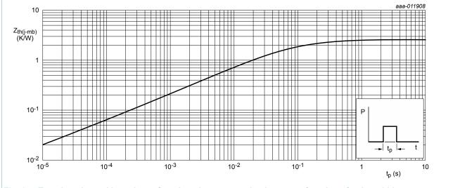
Transient thermal impedance from junction to mounting base as a function of pulse width
