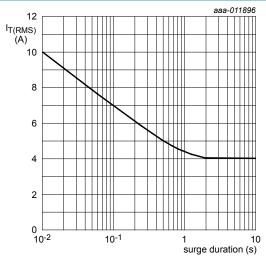
$f = 50 \text{ Hz}; T_{mb} = 113 \text{ }^{\circ}\text{C}$
