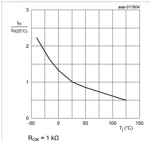
Fig. 9. Normalized holding current as a function of
