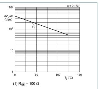
Fig. 12. Critical rate of rise of off-state voltage as a function of junction temperature; typical values
