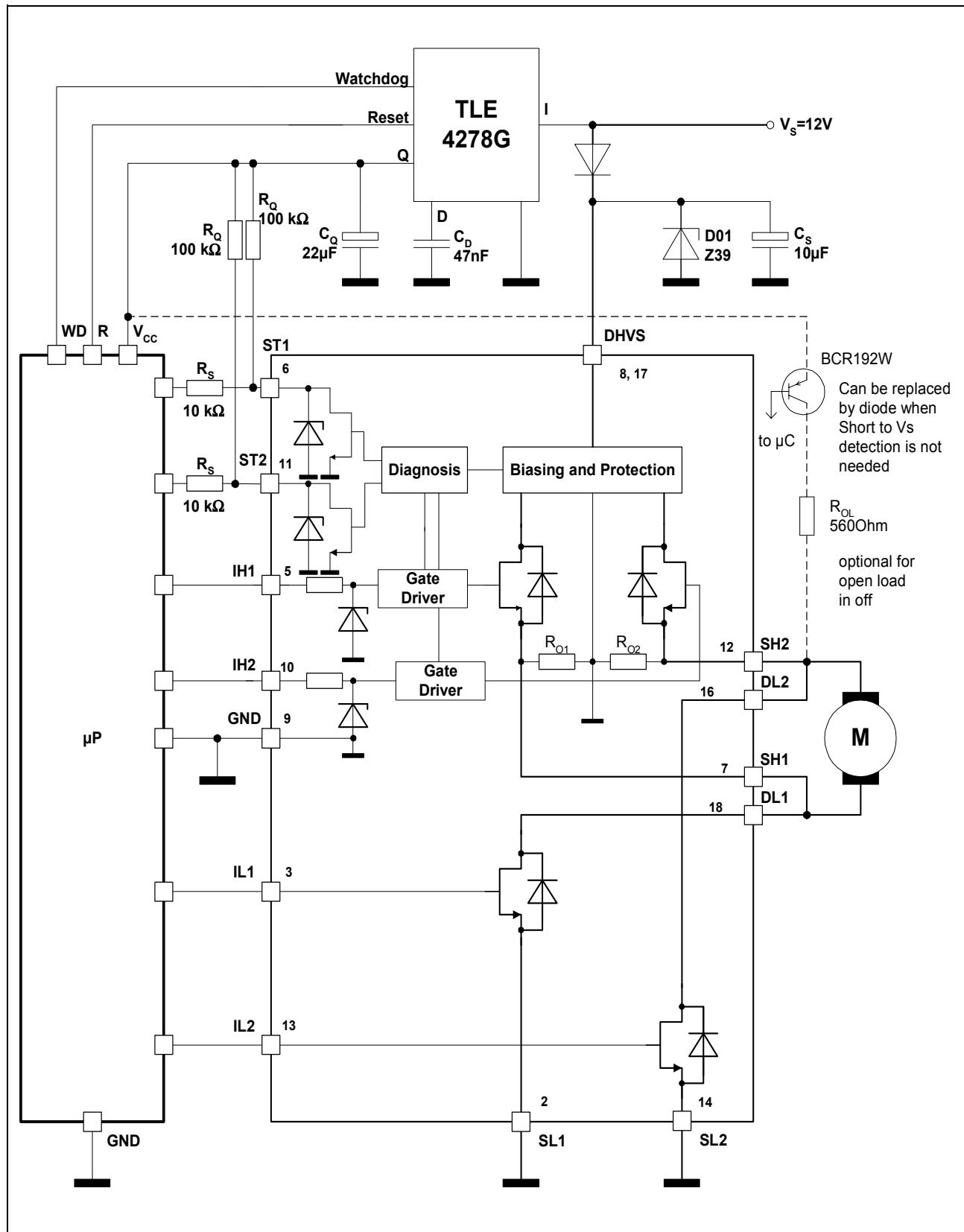
**Figure 5: Application Circuit**
