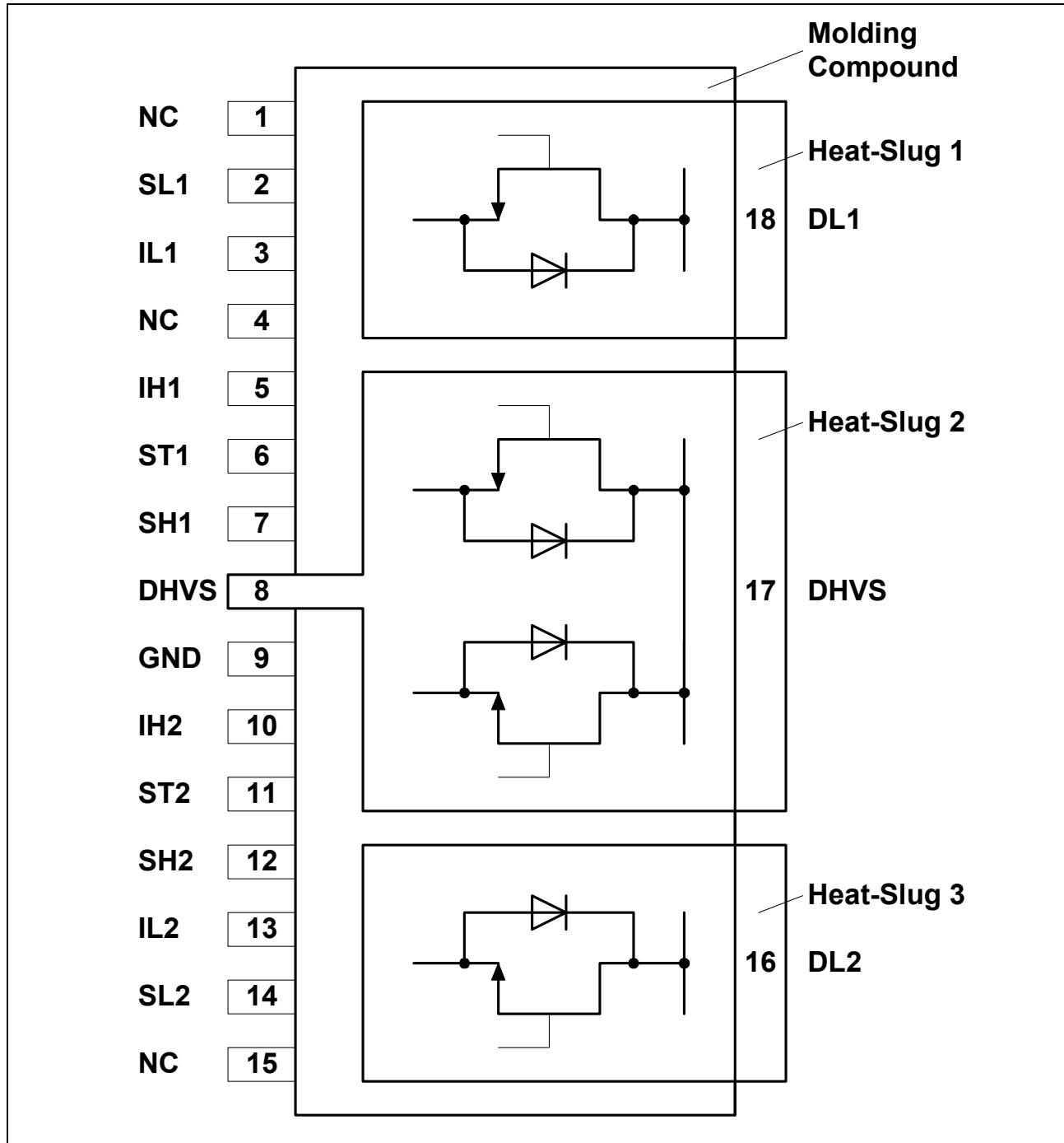
Figure 1: Pin Assignment
