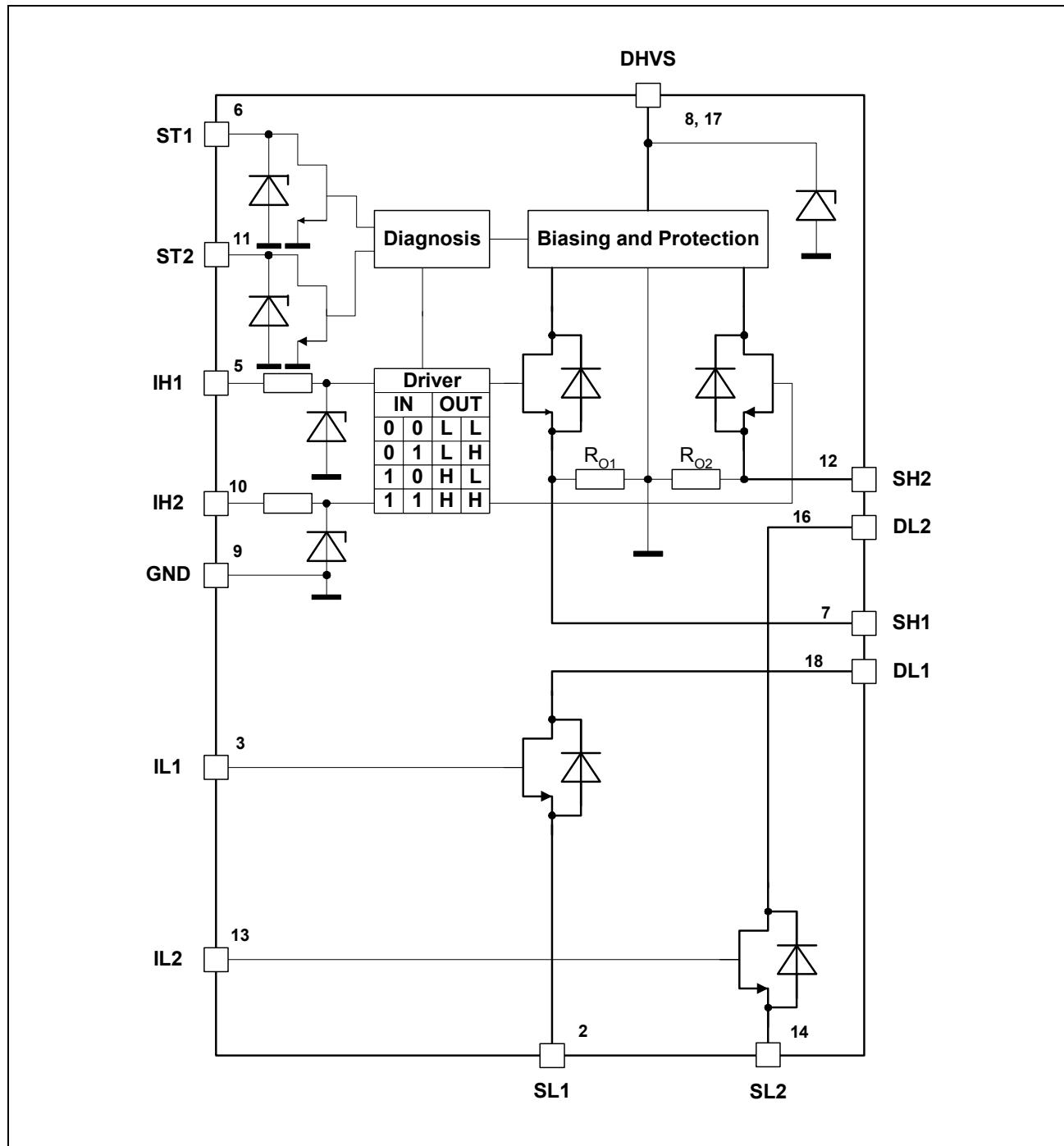
Figure 2: Block Diagram
