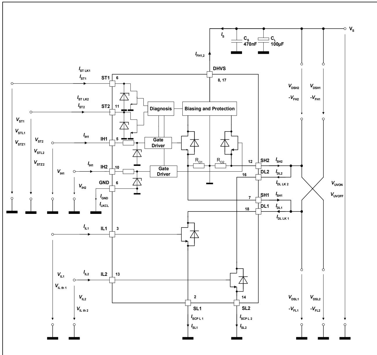
**Figure 4: Test Circuit**
