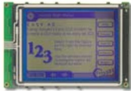
MK-AOB3202405B (STN Negative, Blue, Transmissive)
