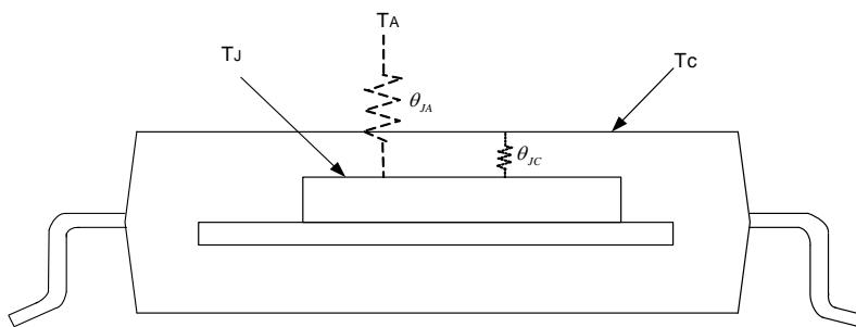
Notes: 5. θ<sub>JA</sub> should be confirmed with what heat sink thermal resistance. If no heat sink contacting, θ<sub>JA</sub> is almost the same as θ<sub>Jc</sub>.
