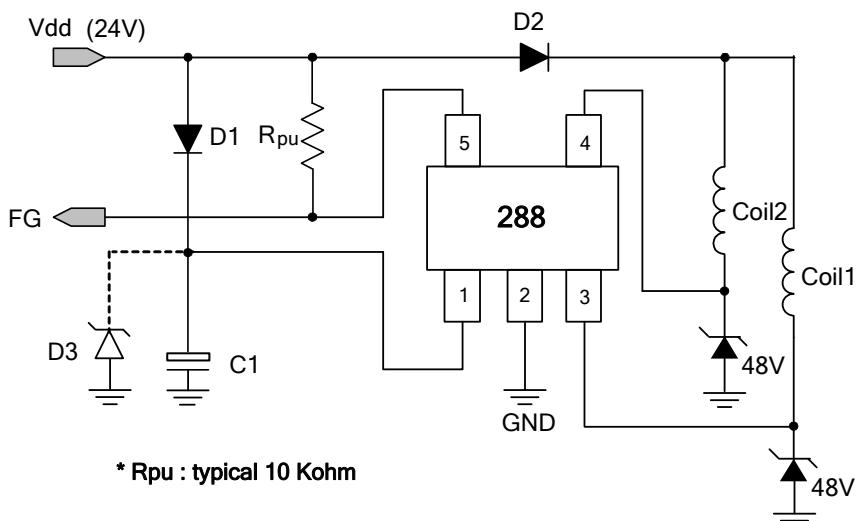
Note: The optional Capacitor C1 and Diode D3 are for power stabilization. C1 is recommended to be E-Cap.,  $1\mu F/25V$ ; D3 is recommended to be Zener Diode,  $V_Z = 27V$ . Which C1 and D3 value need to be fine tuned to optimize design for different coils and power suppliers.
