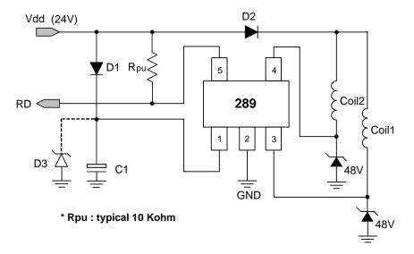
Note: The optional Capacitor C1 and Diode D3 are for power stabilization. C1 is recommended to be E-Cap., luF/25V; D3 is recommended to be Zener Diode, V<sub>Z</sub>=27V. Which C1and D3 value need to be fine tuned to optimize design for different coils and power suppliers.
