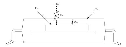
5.  $\theta_{JA}$  should be confirmed with what heat sink thermal resistance. If no heat sink contacting,  $\theta_{JA}$  is almost the same as  $\theta_{JC}$ . Notes:
