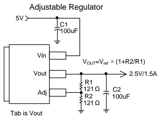
Note:  $V_o = V_{RE}_F * \left(1 + \frac{R_2}{R_1}\right)$
