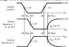
Waveform 1 is for an output with internal conditions such that the output is LOW except when disabled by the output control. Waveform 2 is for an output with internal conditions such that the output is HIGH except when disabled by the output control. All input pulses have the following characteristics: frequency = 10 MHz,  $t_r = t_f = 2$  ns,  $Z_O = 50\Omega$ . The outputs are measured one at a time with one transition per measurement.
