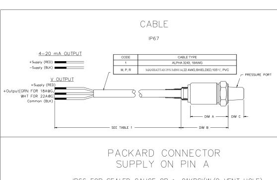
IP66 FOR SEALED GAUGE OR >=01KPSI(W/O VENT HOLE)
