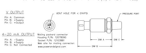
Datasheet of M5131-000005-01KPG - SENSOR PRESSURE 1KPSIG ANALOG
