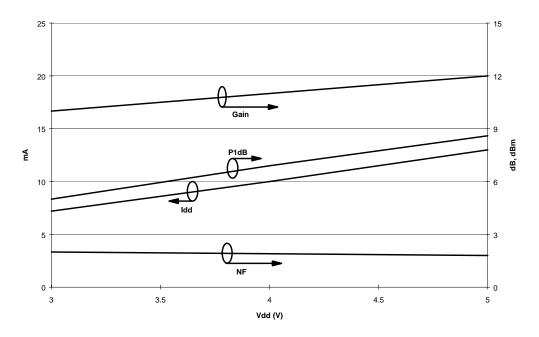
**Typical Characteristics - V<sub>DD</sub>=5.0V**
