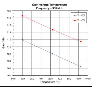
Datasheet of RF2304TR7 - IC AMP GEN-PURP LOW-NOISE 8-SOIC
