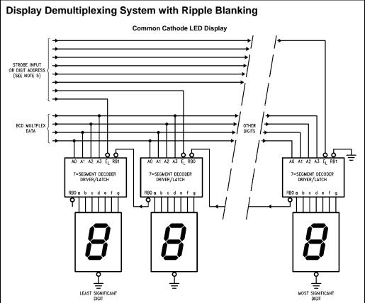
Note: Digit address data must be non-overlapping. Standard TTL decoders like the 9301, 9311, 7442 or 74155 must be strobed, since the address decoding glitches could cause erroneous data to be strobed into the latches.
