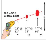
Use the Fluke 68 and 68IS within 8 m (25 ft.) of the intended target. At greater distances, the measured area will be larger (approximately the distance divided by 50).
