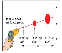
Use the Fluke 66 within 5 m (15 ft.) of the intended target. At greater distances, the measured area will be larger (approximately the distance divided by 30).
