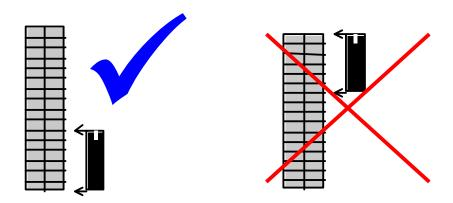
For 3 pin TO220 or TO92 packages, insert the IC in pins 6, 7 and 8 (lower left) of the socket with the metal tab or flat side facing to the right.
