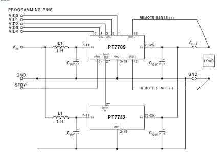
External Capacitors: The PT7743 requires a minimum ouput capacitance of 330µF for proper operation. The PT7743 also requires an input capacitance of 1500µF, which must be rated for a minimum of 1.4Arms of ripple current. For transient or dynamic load applications additional capacitance may be required. For further information refer to the application note regarding capacitor selection for the this product.
