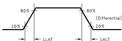
Figure 4. DS90C365A (Transmitter) LVDS Transition Times
