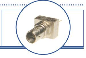
The OPF397 family fiber optic transmitters are high performance devices packaged for data communication links. This transmitter is an 850nm GaAlAs LED and is specifically designed to efficiently launch optical power into fibers ranging in size from 50/125µm up to 200/300µm diameter fiber. Multiple power ranges with upper and lower limits are offered which allows the designer to select a device best suited for the application.
