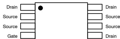
Figure 2. Pinouts for Single Die TSSOP
