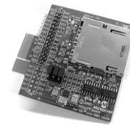
The PICTail Daughter Board for SD and MMC cards (AC164122) is a universal board that interfaces the Secure Digital (SD) and Multi-Media Card (MMC) to the Serial Peripheral Interface (SPI) bus of the microcontroller. This PICTail board is designed to operate with a multitude of demonstration boards, including all those having PICTail signals, those with PICTail Plus signals (utilizing the card-edge connectors like the Explorer 16), and those with non-standard PICTail signals.
