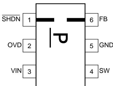
Note: This IC could be destroyed in some case if amounted in 180° inverse direction.
