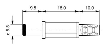
Cable diameter max. 4.0 mm
