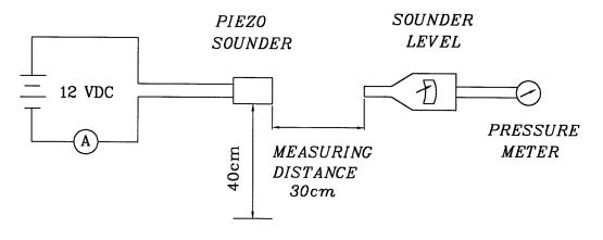
S.P.L. Measuring Circuit Mic: RION S.P.L. meter UC30 or equivalent S.G.: Hewlett Packard 33120A function gernerator or equivalent
