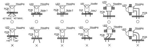
" ( ) " Correct mounting method " imes " Incorrect mounting method
