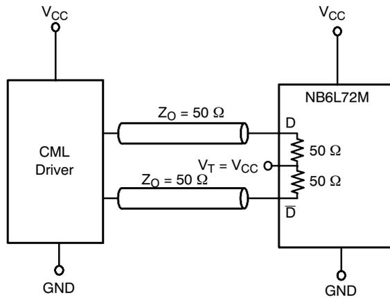
**Figure 12. Standard 50 ohm Load CML Interface**
