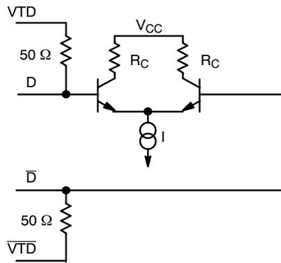
**Figure 3. Input Structure**
