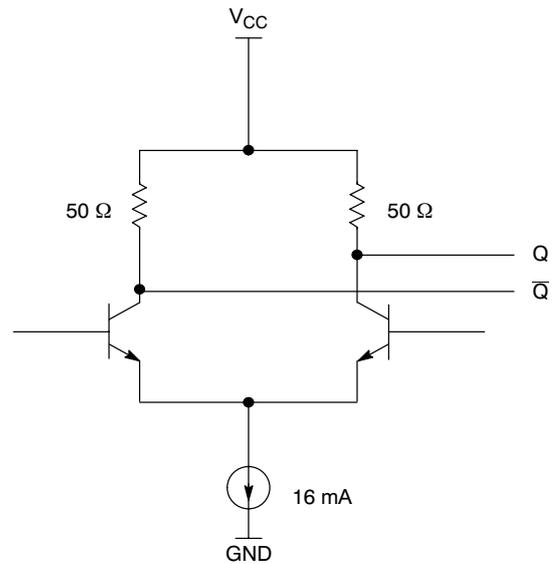
Figure 16. CML Output Structure
