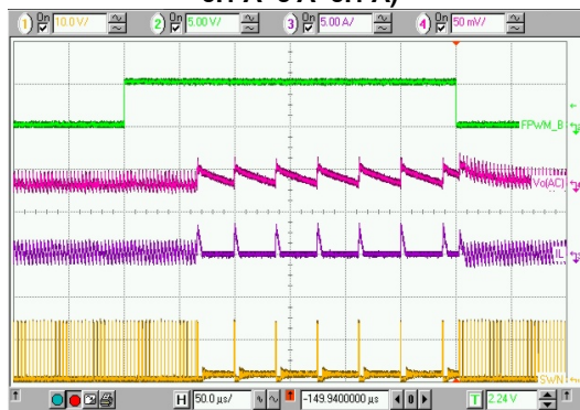
Top: FPWM#, FPWM# Signal, (5V/div) Middle 1: Vo2, CH2 Output Voltage Ripple, (50mV/div) Middle 2: iL2, CH2 Inductor Current, (5A/div) Bottom: SWN2, CH2 Switching Node Voltage, (10V/div) Time: 50μs/div
