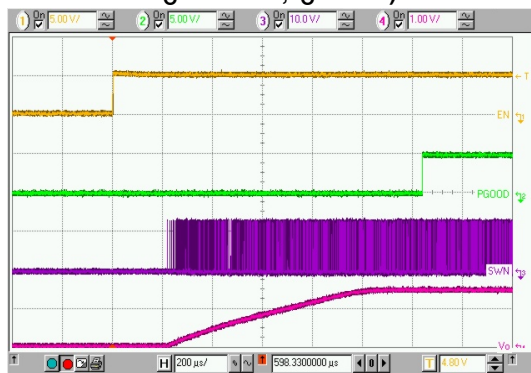
Top: EN1, CH1 Enable Signal, (5V/div) Middle 1: PGOOD1, CH1 Power Good Signal, (5V/div) Middle 2: SWN1, CH1 Switching Node Voltage, (10V/div) Bottom: V_{O1} , CH1 Output Voltage, (1V/div) Time: 200μs/div
