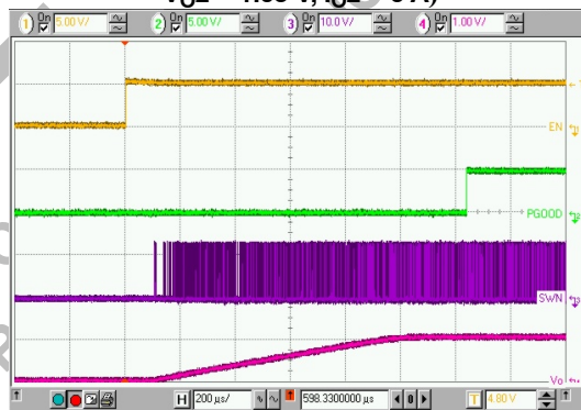
Top: EN2, CH2 Enable Signal, (5V/div) Middle 1: PGOOD2, CH2 Power Good Signal, (5V/div) Middle 2: SWN2, CH2 Switching Node Voltage, (10V/div) Bottom: V_{O2} , CH2 Output Voltage, (1V/div) Time: 200μs/div
