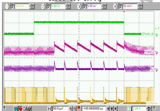
Top: FPWM#, FPWM# Signal, (5V/div) Middle 1: Vo1, CH1 Output Voltage Ripple, (50mV/div) Middle 2: iL1, CH1 Inductor Current, (5A/div) Bottom: SWN1, CH1 Switching Node Voltage, (10V/div) Time: 50μs/div
