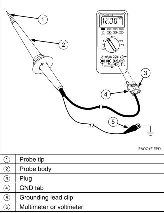
Figure 1. 80K-15 Electronic Air Cleaner Probe
