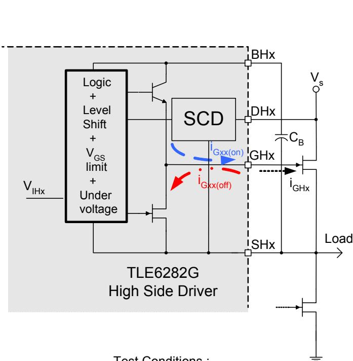
This figure represents the simplified internal circuit of one high side gate drive. The drive circuit of the low sides looks similar.
