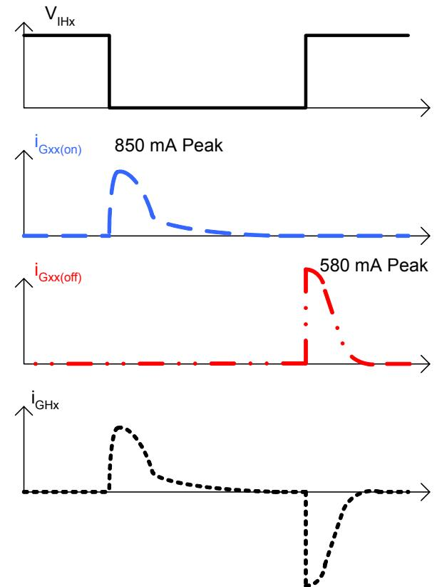
This figure illustrates typical voltage and current waveforms of the high side gate drive; the associated waveforms of the low side drives look similar.
