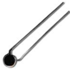
143 Series, 5,08 mm [0.2 in] disc thermistor with leads, 30,000 Ohm resistance, ±10.0% tolerance, 25/85 BETA = 4261
