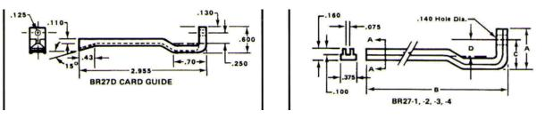
Description Secure connection Rugged support of 0.062" thick Free standing circuit boards For application in which space is premium Several size and styles available Aluminium alloy construction Mounting hardware included { HD55 Hardware Kit } TS169 " T-Strut " mounting rail available BR27D
