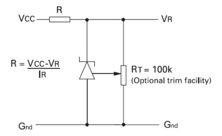
This circuit will allow the reference to be trimmed over a wide range. The device is specified over a ±5% trim range.
