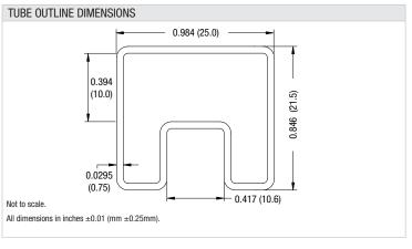
All dimensions in inches  $\pm 0.01$  (mm  $\pm 0.25$ mm). All pins on a 0.1 (2.54) pitch and within  $\pm 0.01$  (0.25) of true position.
