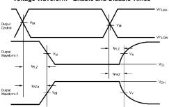
Output Waveform 1 is for an output with internal conditions such that the output is LOW except when disabled by the control output Output Waveforms 2 is for an output with internal conditions such that the output is HIGH except when disabled by the control output
