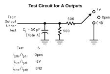
Note A: C<sub>L</sub> includes probes and jig capacitance.
