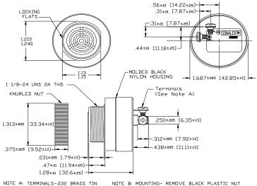
NOTE A: TERMINALS-.032 BRASS TIN PLATED, TAPPED FOR #6-32 SCREW. TWO #6-32 NICKEL PLATED BRASS SCREWS INCLUBED. WILL ACCEPT 1/4\* QUICK CONNECT. E B: MOUNTING- REMOVE BLACK PLASTIC NUT AND INSERT THREADED FRONT THROUGH 1.25' HOLE PUNCHED IN PANEL, IF DRIENTATION IS NEEDED, NOTE LOCKING FLATS ON DRAWING, SCREW NUT BACK ON. DO NOT OVERTIGHTEN.
