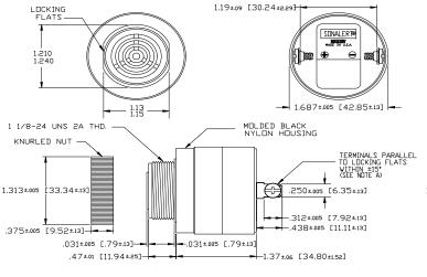
NOTE A: TERMINALS-.032 BRASS TIN PLATED, TAPPED FOR #6-32 SCREW. TWO #6-32 NICKEL PLATED BRASS SCREWS INCLUDED. WILL ACCEPT 1/47 QUICK CONNECT. NOTE B: MOUNTING- REMOVE BLACK PLASTIC NUT AND INSERT THREADED FRONT THROUGH 1.25' HOLE PUNCHED IN PANEL, IF ORIENTATION IS NEEDED, NOTE LOCKING FLATS ON DRAWING. SCREW NUT BACK ON. DO NOT OVERTIGHTEN.
