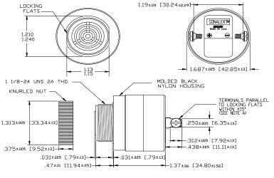
NOTE B: MOUNTING- REMOVE BLACK PLASTIC NUT AND INSERT THREADED FRONT THROUGH 1.25' HOLE PUNCHED IN PANEL, IF ORIENTATION IS NEEDED, NOTE LOCKING FLATS ON DRAWING. SCREW NUT BACK ON. DO NOT OVERTIGHTEN.
