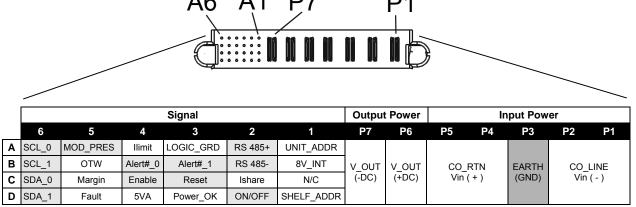
Connector is viewed from the rear positioned inside the power supply.
