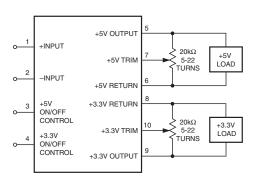
Figure 2. Trim Connections Using A Trim Pot
