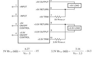
Figure 4. Trim Connections To Increase Output Voltages Using Fixed Resistors
