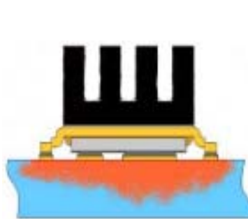
⑩ Mounted on minimum footprint full size board with metalized back and with small clip heatsink. (still air)
