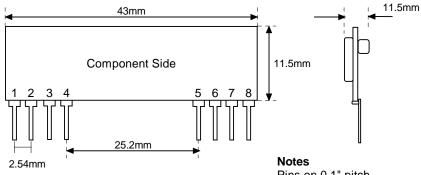
Pins on 0.1" pitch Pin Dims :0.25 x 0.50mm
