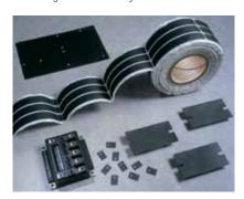
Bergquist Q-Pad 3 eliminates problems associated with thermal grease such as contamination of electronic assemblies and reflow solder baths. Q-Pad 3 may be installed prior to soldering and cleaning without worry. When clamped between two surfaces, the elastomer conforms to surface textures thereby creating an air-free interface between heat-generating components and heat sinks.
