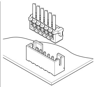
The KR connector features a mounting height as low as 6.9mm and a thickness as thin as 4.8mm (for top entry type). It is suitable for interconnection of a wide range of electronic equipment such as VCRs, video cameras, car stereo systems and communication equipment.
