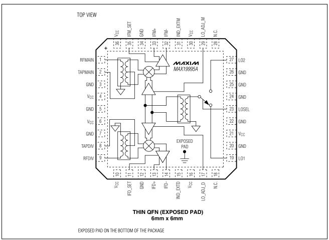
Pin Configuration/Functional Diagram
