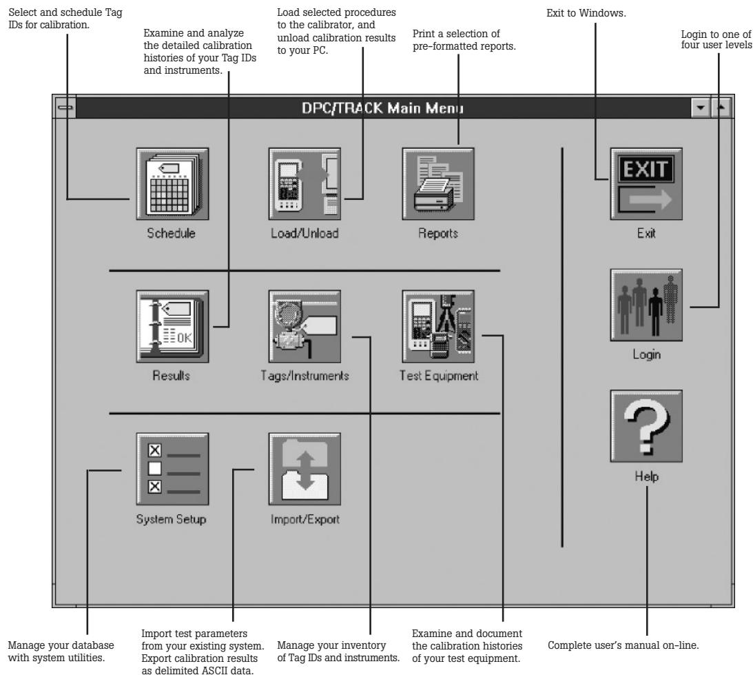
Fluke 700SW DPC/TRACK software includes an instrumentation database that makes it easy to manage your instrumentation, create and schedule tests, load and unload the 743 or 744, print a variety of standard reports, and manage calibration data.
