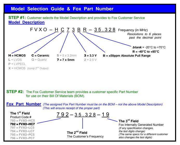
This example, FVXO-HC73BR-35.328 = Voltage Controlled, HCMOS Output, Ceramic, 7 x 5mm Package, 3.3V, ±50 PPM Absolute Pull Range, -40 to +85°C Temperature Range, at 35.328 MHz
