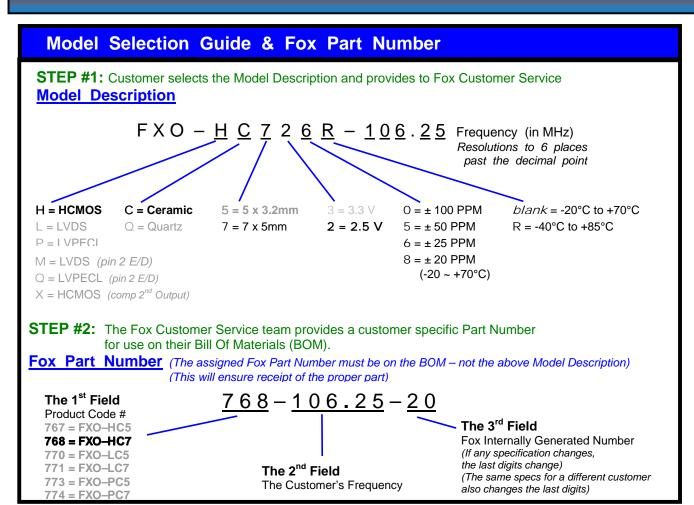
This example, FXO-HC726R-106.25 = HCMOS Output, Ceramic 7 x 5mm Package, 2.5V,  $\pm 25$  PPM Stability, -40 to  $\pm 85$ °C Temperature Range, at 106.25 MHz
