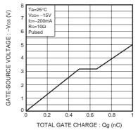
Fig.3 Dynamic Input Characteristics
