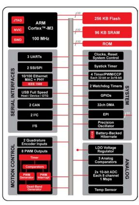
**LM3S9000 Series Block Diagram.** This block diagram shows the superset of features for the LM3S9000 series of microcontrollers.
