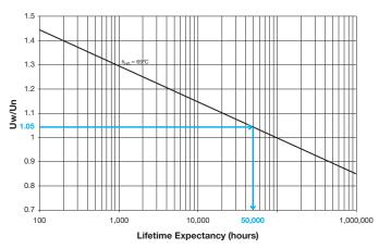
eg: rated voltage 1000V working voltage 1050V ρ = 1.05 ⇒ lifetime 50,000 hours @ 65°C hot spot temperature
